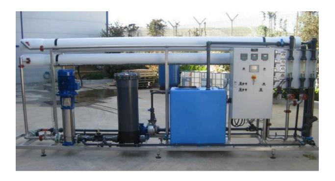
The plant is situated in Czech Republic. Due to the contaminants in raw water, a sophisticated pre-treatment was implemented in order to feed the R.O. membranes with water of suitable quality.
